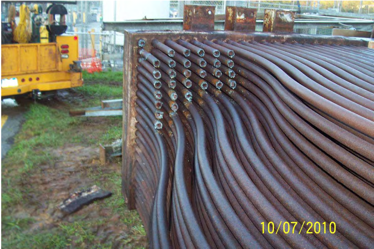
Stainless steel recuperator rods.
